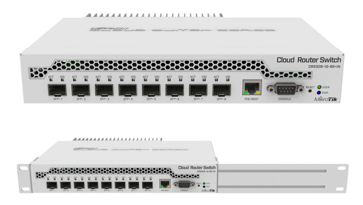
The compact and sleek metallic enclosure also acts as a heatsink, making this device passively cooled no fan noise and no dust accumulation inside. Special rackmount ears for installing unit into the standard rack are provided.
