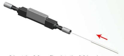
2.Inert the 0.9mm fiber into the 0.9 head of the Body.
