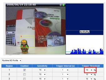
The blue graph on the right side of the image shows how many percent of pixels within the motion detection
