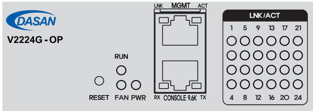
**Figure 4** LEDs on the V2224G-OP
