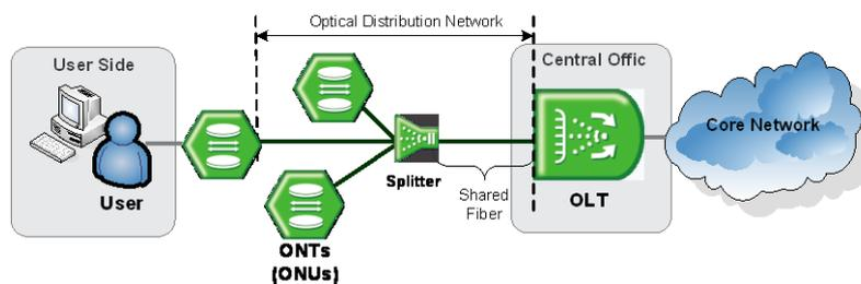
**Figure 5** Optical Distribution Network by PON Architecture
