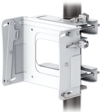
The Precision Alignment Kit is available as an optional accessory for the AF-5G30-S45. It features 15° of azimuth adjustment and 15° of elevation adjustment to enable extremely accurate aiming for optimal PtP link performance.
